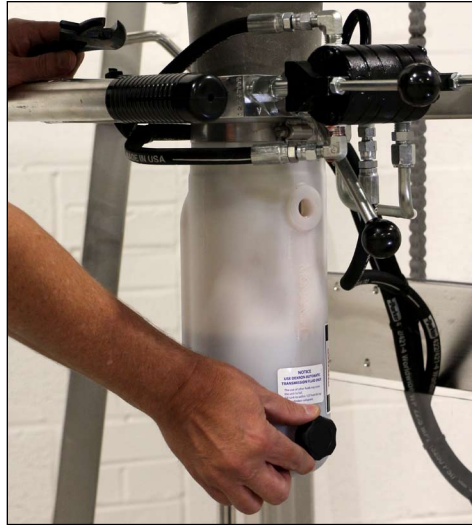
Remove BLACK breather from storage position
